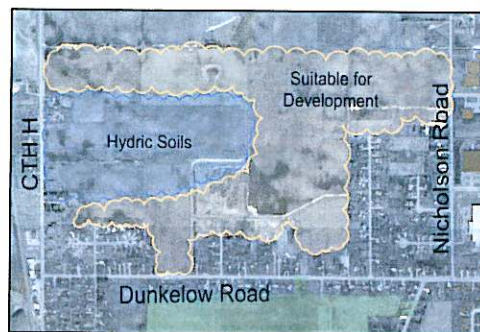
Figure 3-17. Diagrammatic illustration of soil conditions. Before any development occurs in this area, a detailed soils analysis must be completed.
