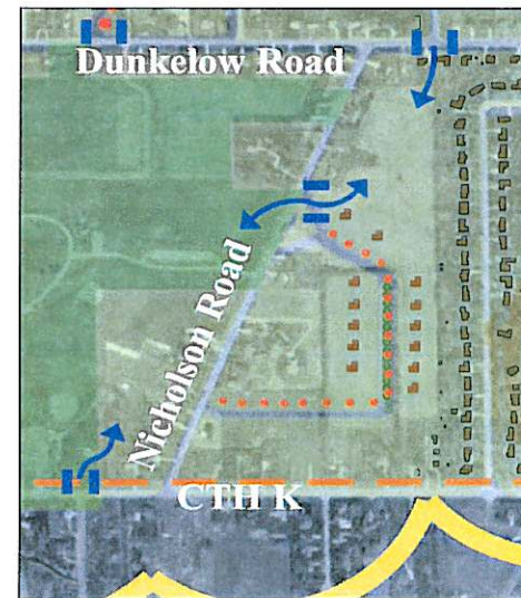
Figure 3-19. Conceptual road alignment for Nicholson Road represented by the larger red dots. For additional key symbols, see Page 39.
